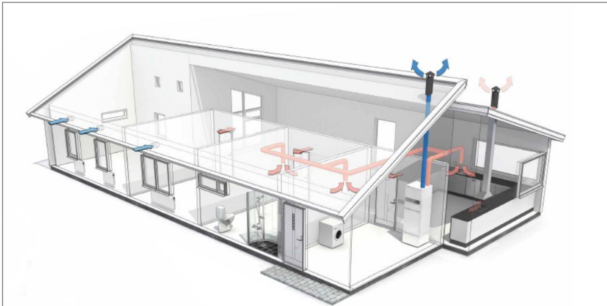
Figure 5 – Typical EAHP flow diagram
