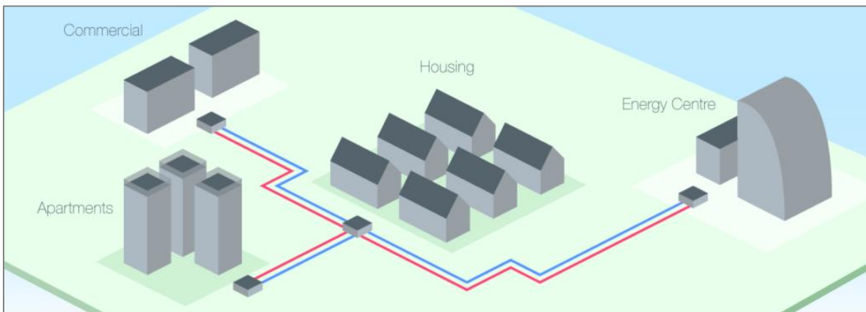
Figure 2 - District heating flow diagram (overview)
