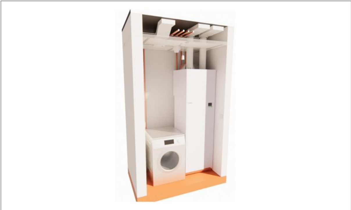
Figure 6 - EAHP Service Cupboard
